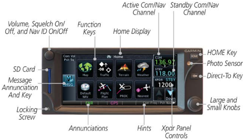
Figure 2 GTN 635/650 Control and Display Layout
