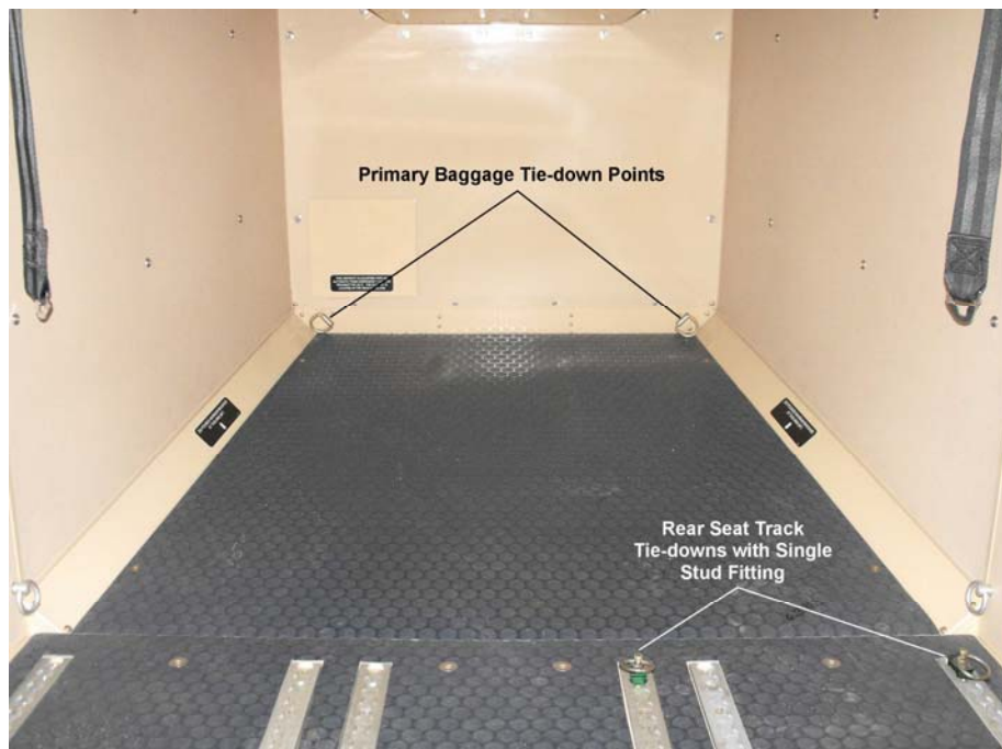
Figure 6-14 Primary Tie-downs in Baggage Compartment
